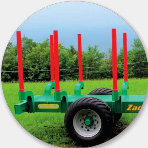
Steel poles, 10 mm thick, from diam. 70 to 90, height 1,50 mt., with fixing screw
