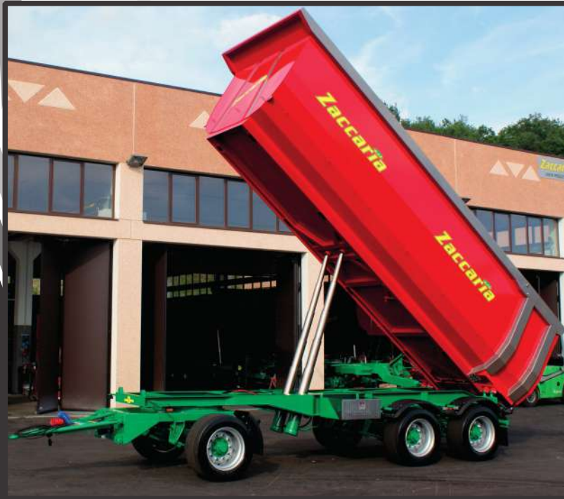
Removable-body trailers with lateral parking stands
